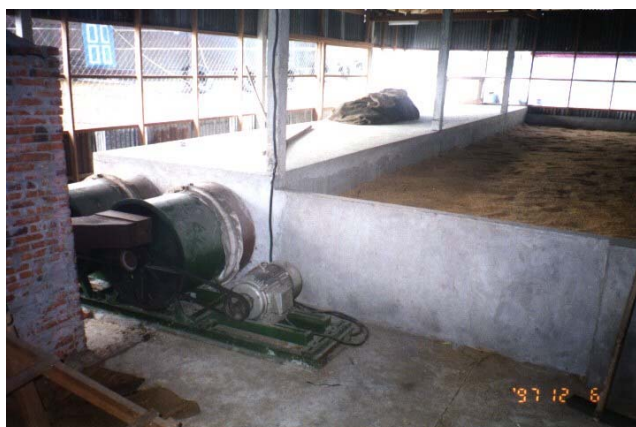
Figure 1: SHG-8 dryer, developed in 1996; over 600 units are now in the Mekong Delta of Vietnam
