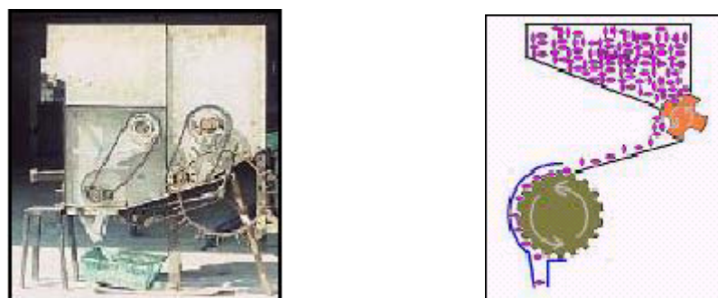
(b) Vertical plate garlic planter and the schematic view.
