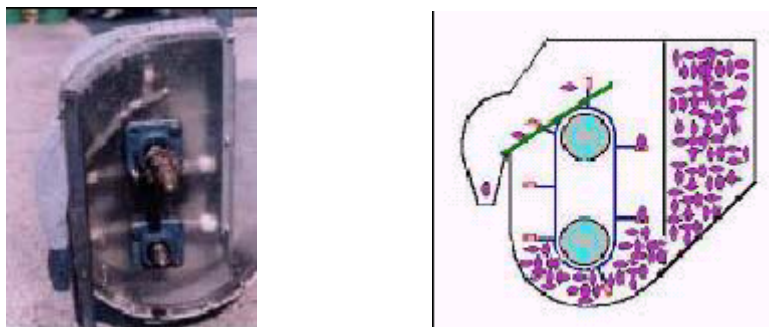
Figure 3: Bucket type metering system.
