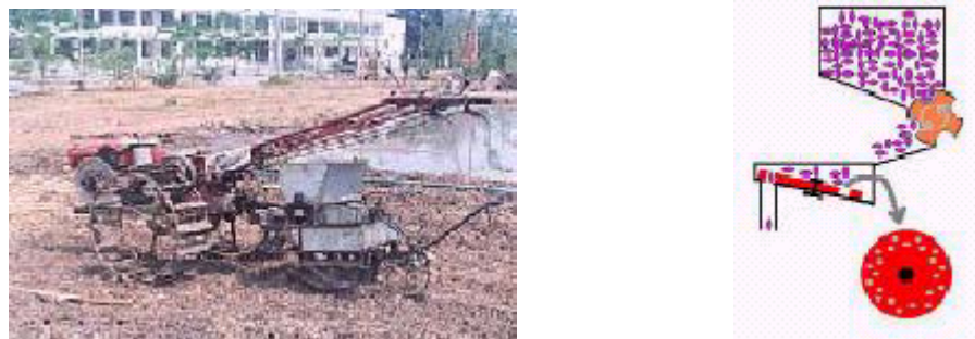
(a)Inclined plate garlic planter and the schematic view.
