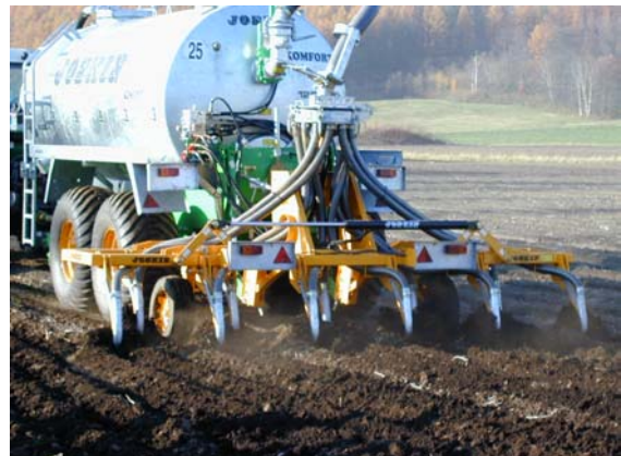
Figures 5: Typical deep injector
